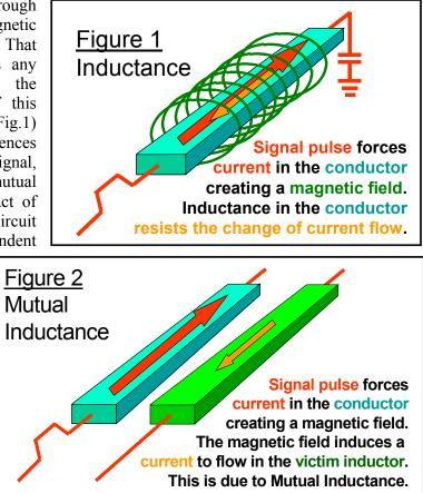
conductor width gets wider, the resistance drops rapidly and the frequency at which inductance shows a significant effect can be lowered to the operating frequencies of today's
