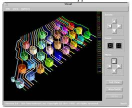
dimensional structures that have perfect ground planes. It cannot be used for structures without ground planes where the 'TEM mode' does not exist. The OEA program, HENRY, uses the partial equivalent element calculation method for extracting inductance. **HENRY** calculates very accurate frequency-dependent inductance models of a full package in just minutes.
