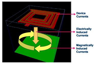
Figure 6. Passive Components must include Self Capacitance, Capacitance to Substrate, High Frequency Skin Effect etc.
