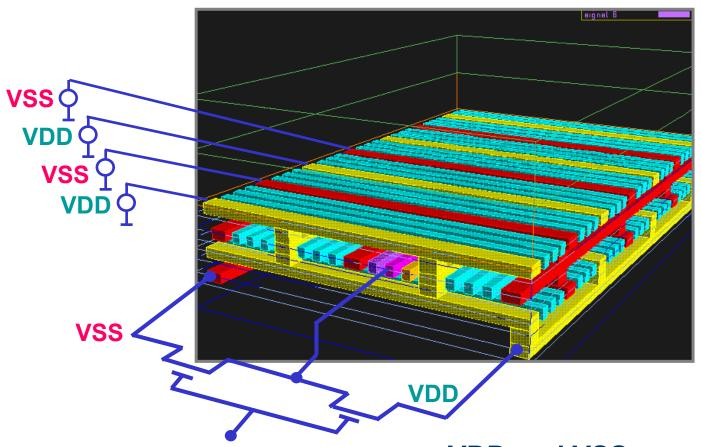
VDD and VSS couple to the signal and have significant inductance and capacitance
