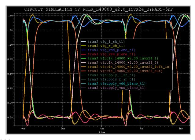
Length =  $4000 \mu$ Width =  $2.0 \mu$ Driver = 24X Inverter Load = 1X Inverter with 50fF Load
