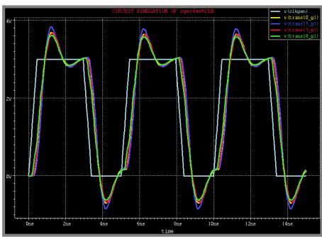
0.45 nS rise and fall times (0 - 3 Volt Transition) Four, 50fF Loads, 200 MHz Clock
