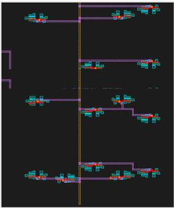
One or more 'Target Nets' are identified in the layout. This can be through an XY,layer, net name, or GDSII Reference file.
