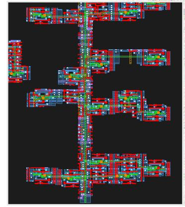
A 3D model is created with a 'Extraction Halo' for capacitance to neighbors. Inductance coupling is determined by a minimum coupling value.
